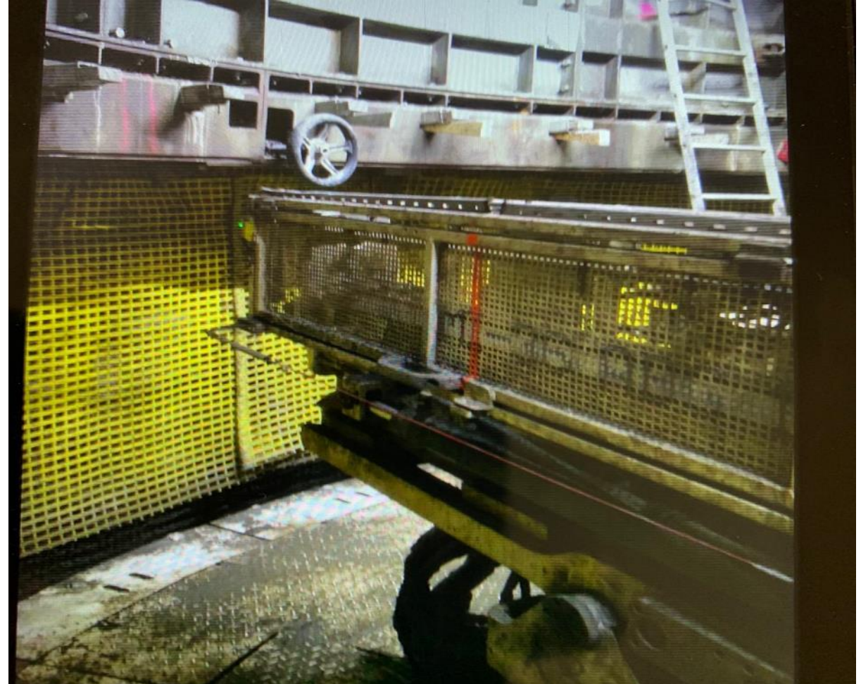
Anchored drill commissioned on deck 2 for installation of ground supports
